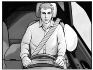
If your vehicle has a driver's side impact air bag it is located in the side of the driver's seatback closest to the door.
